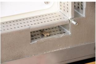
Check the room between the penetration bezel and the inner bezel, which is covered with a plate of acrylic glass, for heavy solings like bullet splinters.
