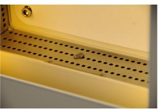
Check the bezel in the penetration area for heavy soilings like bullet splinters.
