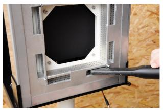
Clean the room between the inner and outer bezel with a soft cloth, a soft brush, compressed air or a vacuum cleaner. Pay attention that you don't scratch the acrylic glass plates on the inner bezel of the measuring frame.
