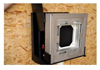
Remove the bullet trap cover from the left side of the bullet trap by pulling it up.
