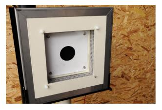
Put the four white nuts back onto the screws and tighten it.
