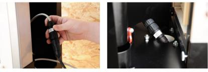
connect the LED lighting power adapter (C1) with the put the connected cable measuring frame cable (D2) and tie it up into the hole
