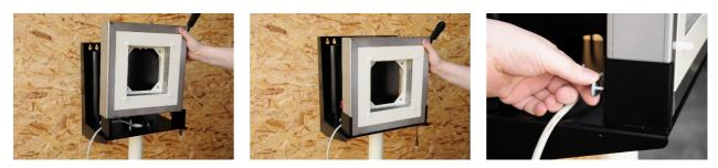
put the measuring frame (C3) into the bullet trap and fix it with the screws on the back
