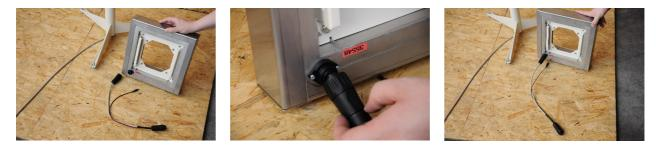
connect the LED lighting power adapter (C1) with the measuring frame (C3) and tie it up
