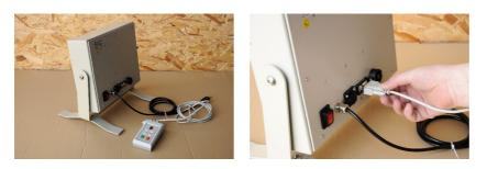
connect the shootmaster control console (D1) to the MC5CPC2 compact control PC (D3) an fix it
