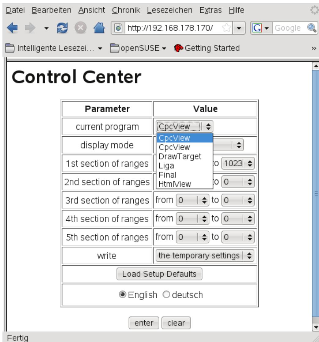
The display program can be chosen, with which the Display Controller starts at every reboot. The Display Controller contains five different display programs.
